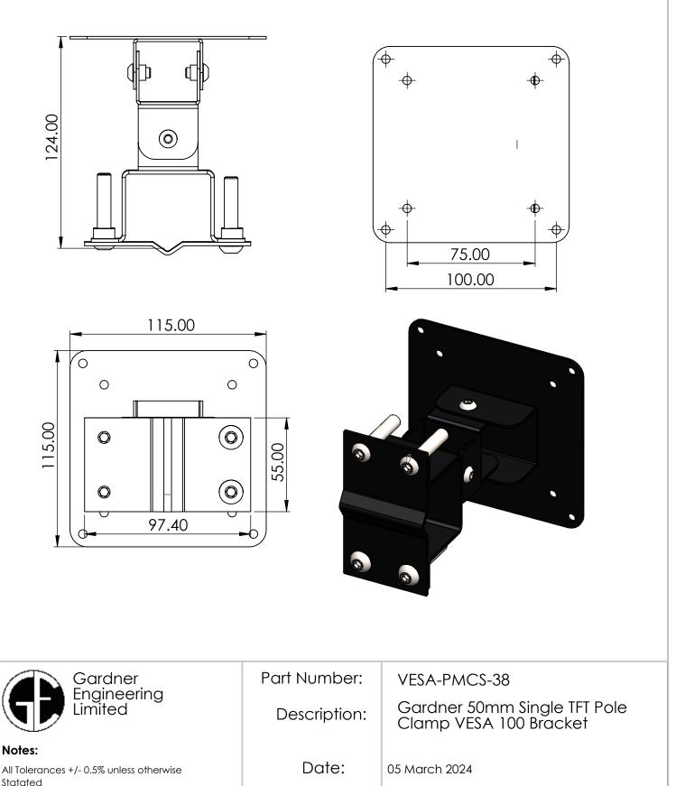
All Measurements are Raw Materials Only and allowances are needed for Welding Tracks & any additional coatings such as Powder Coating / Spray Paints Etc
